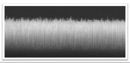
*Figure 1:* Nanomolecular SiO2 crystalline-like structures visualized under high powered electron microscopy. Once dried onto a treated surface, the structures covalently bond to the underlying base substrate, creating a newly modified, antimicrobial, protective surface barrier.
